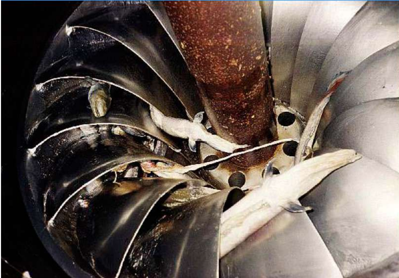
Turbine clogged with eels. Note eel skin stretched across shaft. Photo: Alex Haro, Ph.D. , S. O. Conte Anadromous Fish Restoration Center Presentation- Fish Passage in the Northeast: Old Problems, New Solutions U.S.G.S., Biological Services
